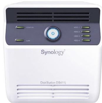
Choose a NAS device that uses **active cooling** (i.e. it uses a fan) instead of **passive cooling**. Thermal stress kills hard drives. It causes damage to the electronics onboard, causes failure of mechanical components and can induce a phenomenon known as the super-paramagnetic effect to corrupt your data. From our NAS data recovery experience, NAS drives that only use active cooling are much likely to be damaged by thermal stress.
